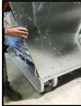
**STEP 76:** Tek screw rain guards to feeder.
