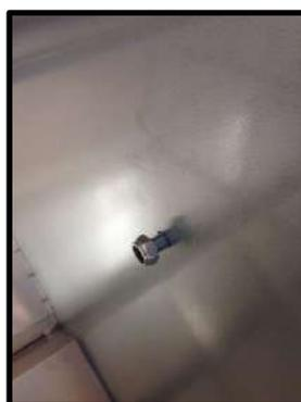
**STEP 47:** Put nut on inside of the feeder.
