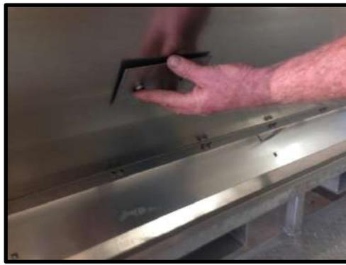
**STEP 38:** Attach supports to divider. Plate is to go onto the outside.
