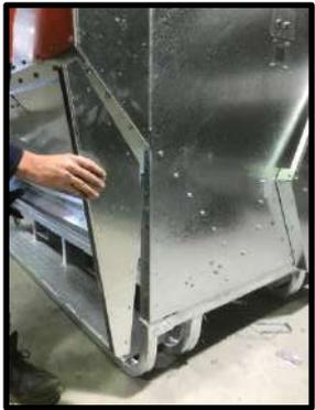
**STEP 75:** Place rain guards on all 4 corners of feeder (There is left and right).
