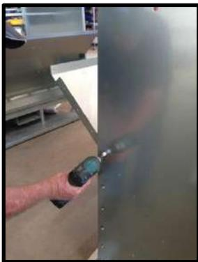
**STEP 31:** Attaching divider to end.
