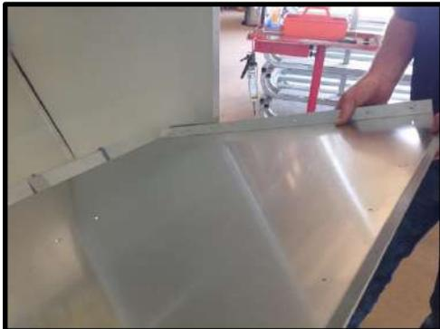
**STEP 28:** Slide dividers through slot in end.
