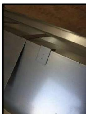
**STEP 20:** Secure angle pieces to base. The letter 'T' must be on top of the other angle.
