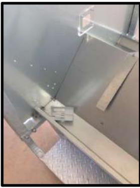
**STEP 25:** Adjuster bracket (Left and right).
