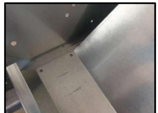
**STEP 12:** Fit base to ends. Line up holes.
