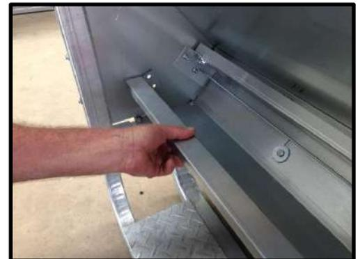
**STEP 54:** If attaching ad-lib pieces line up with the two holes on the ends.
