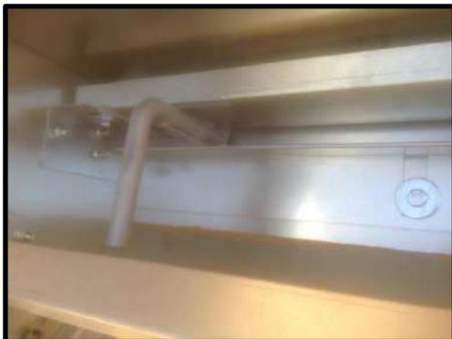
**STEP 52:** Set adjusters so upper adjuster 15mm from bottom to base, 20mm from lower adjuster to upper. This will give approx.. 300gm/day.
