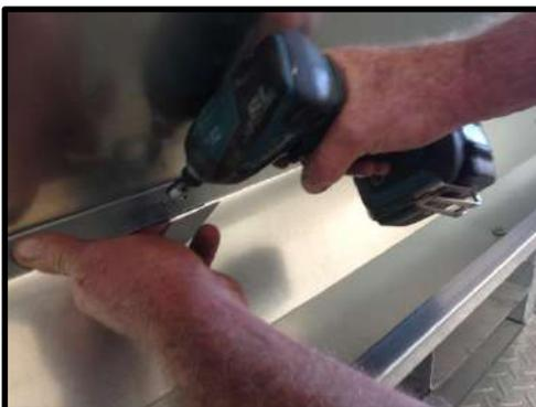
**STEP 34:** Attaching straps to bottom of dividers.
