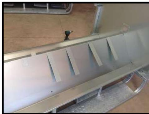
**STEP 23:** Lay out straps on top of base.
