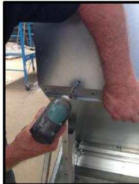
**STEP 68:** Tek screw second hole from the end. Do not do first hole first.
