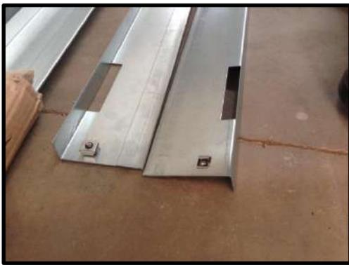
**STEP 49:** Attach cage nuts to upper adjusters. One each end (Note which way the cage nut is attached).
