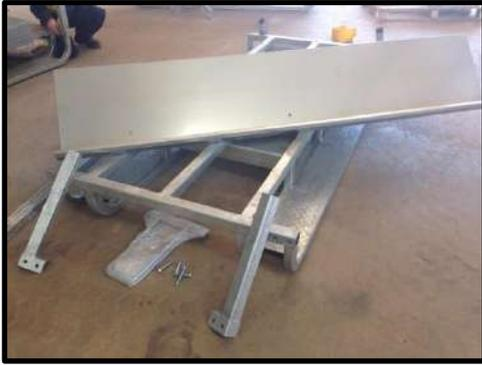
**STEP 1:** Lay posts out on each corner (Left and right) and base onto frame and lid hinges.
