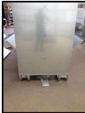
**STEP 32:** Both dividers in place. Ensure all holes fitted with tek screws.
