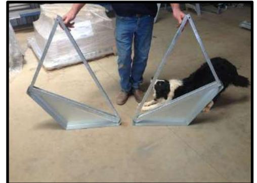
**STEP 45:** Always remember there is a left and a right side, so fit lid ends alternatively to lid RHS hinge.
