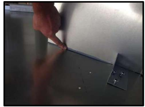
**STEP 27:** Selastic gap between the base and the end (Do not selastic below adjuster bracket). Tighten.
