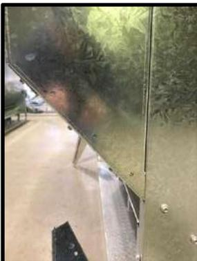
**NOTE:** Do not tek screw these 3 holes. These will be done when rain guards are fitted.
