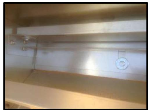
**STEP 51:** Attach bottom adjuster (3 slots in adjuster to the base). Bolt then large washer.
