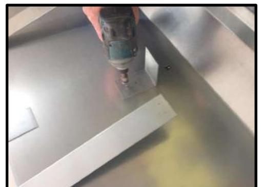
**STEP 21:** The two holes in the base are for the angle pieces.
