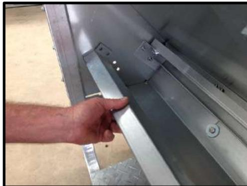
**STEP 53:** Attach bottom adjuster (Has 3 slots).
